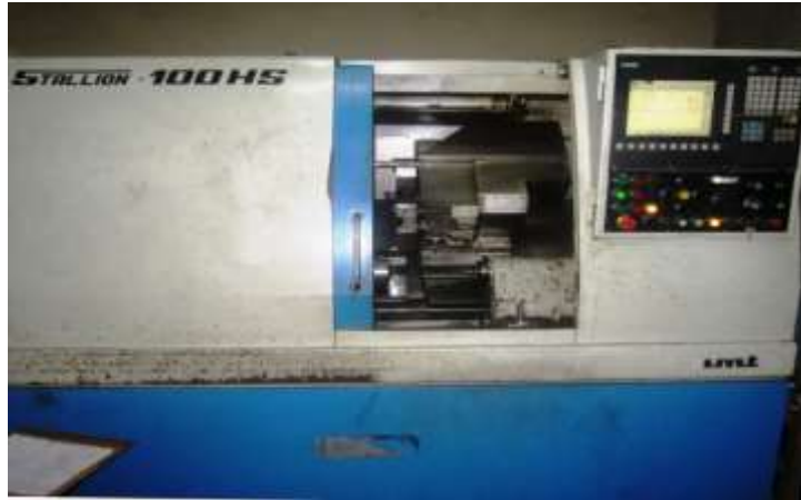
Figure 1: CNC Lathe machine (courtesy: R & D Centre for bicycle and sewing machine, Ludhiana)
